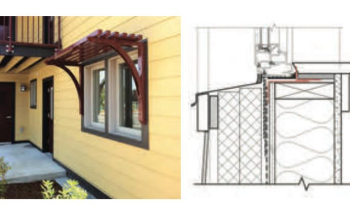
Passive House is a certification that boasts 70% better than code for overall energy performance. From the wall section on the left, the Passive House building has a much thicker wall that consists of more exterior insulation than the Earth Advantage building.
